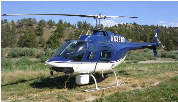
Figure 2 – Bell Jet Ranger equipped with a thermal infrared radiometer. The sensor is contained in a composite fiber enclosure attached to the underside of the helicopter and flown longitudinally along the stream channel.
